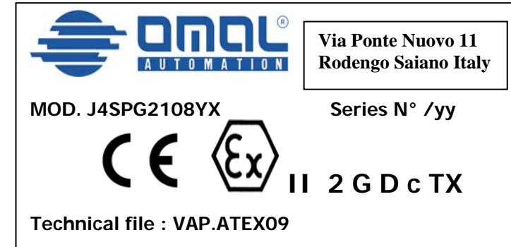
No information about room temperature and process fluid maximum temperature is provided in the ATEX label as it is already marked on the valve body or listed in the technical documents supplied to the User/Safety Instructions.
